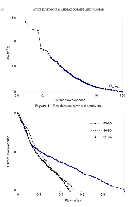
Figure 5 Close-up of the flow duration curve for different drainage period
